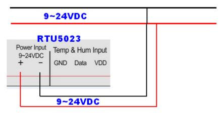
In this condition, the RTU5023 was powered on by the 9~24VDC directly
